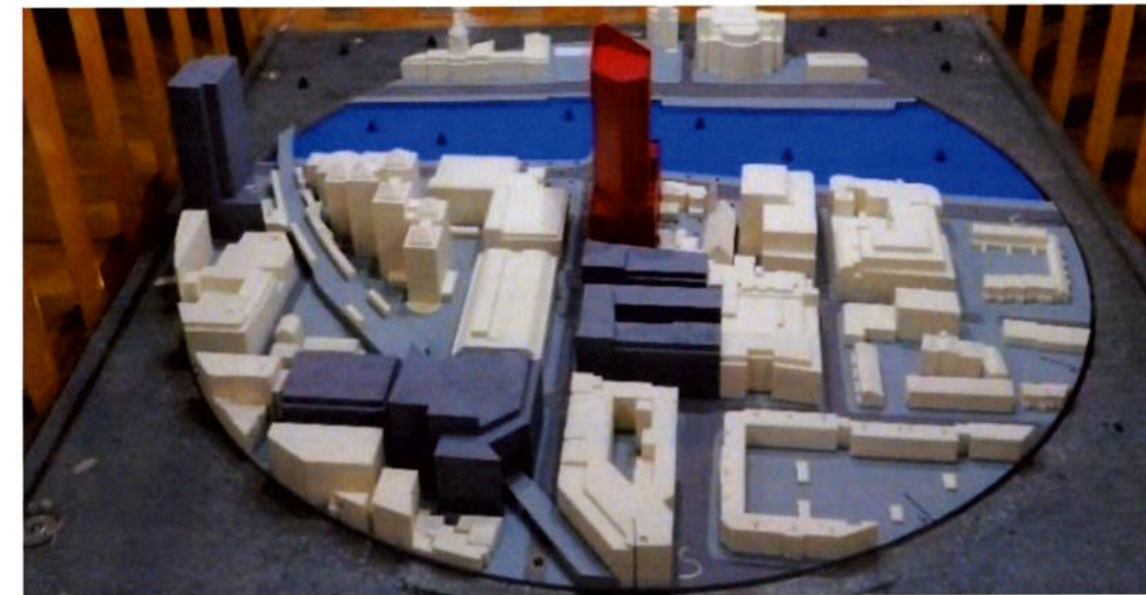
Figure 83. 1;250 model of proposed development in the BRE wind Tunnel ( view from South)
